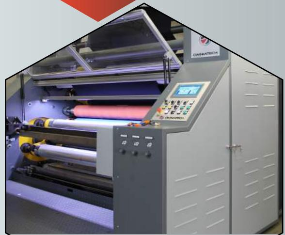
Bonding line with 3 engraved cylinders and cleaning station
