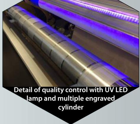
Detail of quality control with UV LED lamp and multiple engraved cylinder
