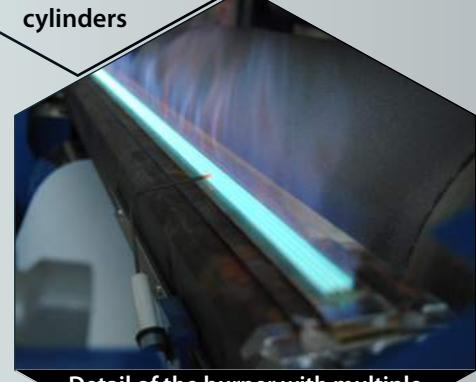
Detail of the burner with multiple nozzles for high precision applications
